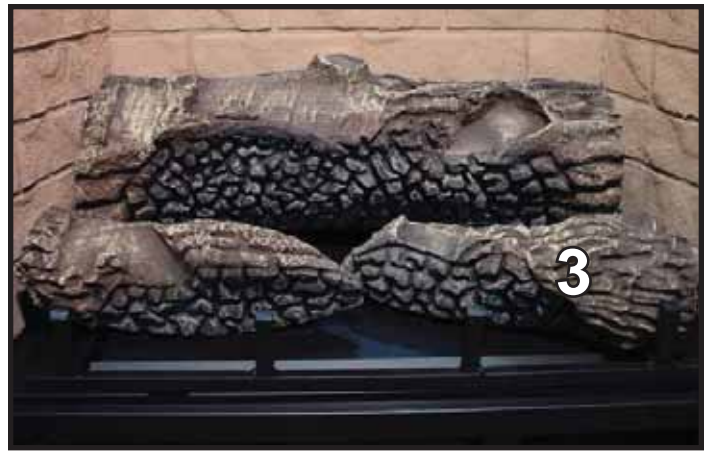
LOG #3 (SRV340-703): Position log #3 by locating its slot over the tab on the front right of the burner. Push the right side forward against the right grate tine.
